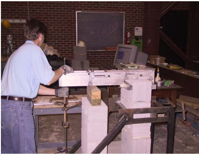
Figure 3 - Proposed Bond Wrench With Couplet Under Test (Note the left stack of blocks and wood were used to catch the arm after failure)
