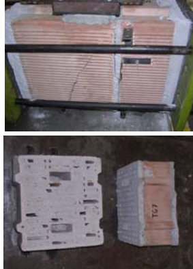
Figure 2 – Test of sliding along a mortar joint: failure of the unit (above), failure of the joint (below)
