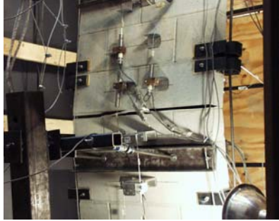
Figure 3 - Photograph of Wall PC6-150-R During Testing
