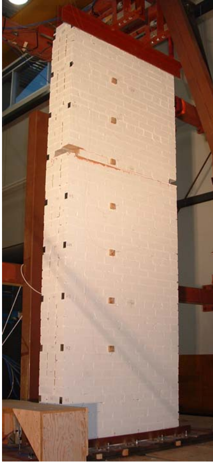
Figure 8 - Good Quality Wall with Crack Formed at Header 6 (Test 4)
