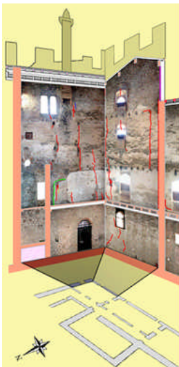
Figure 5 - Avio Castle. Crack pattern survey of the Tower
