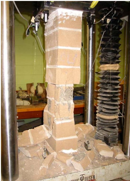
Figure 3 - Clay prism after testing
