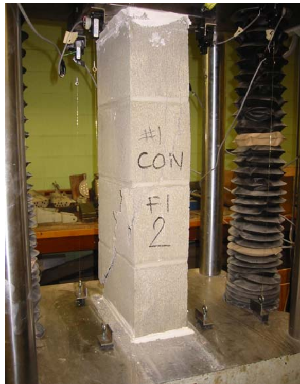
Figure 4 – Concrete prism after testing
