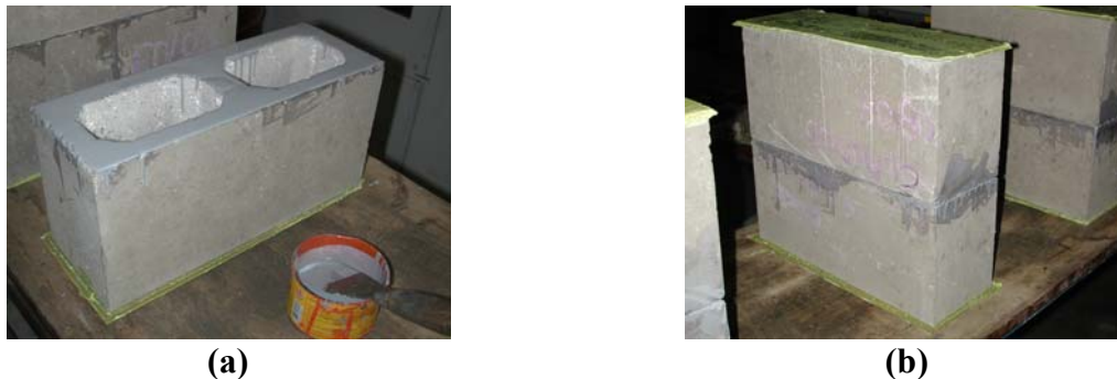
Figure 2 – Hollow concrete block with a thin layer fully bedded (a) and a prism with two blocks (b).
