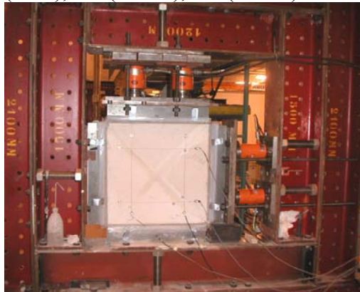
Figure 3 - Test rig and hydraulic system Figure 4 - Loading scheme and LVDT positions
