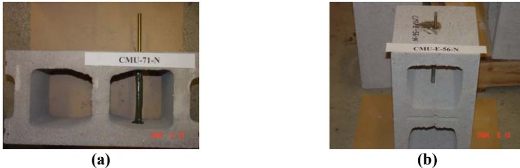
**Figure 7- Anchor Placement in Standard Hollow Concrete Block**
