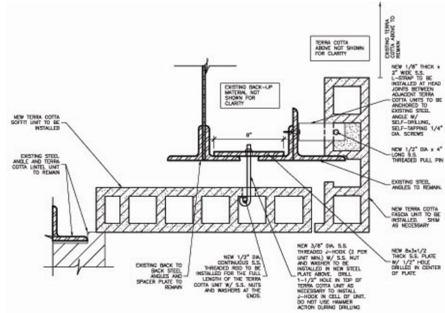
**Figure 7 - Typical cracked terra cotta soffit units (left), new hung soffit detail (right)**
