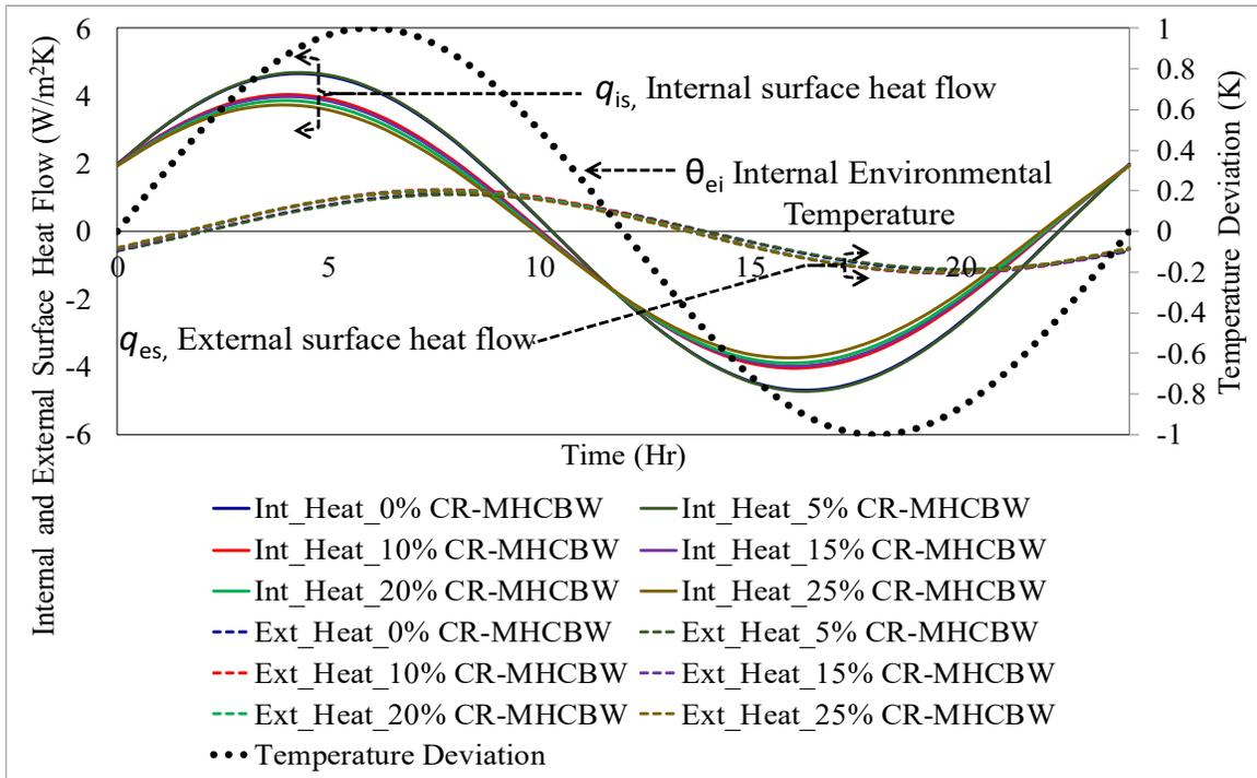
**Figure 2: Surface Heat Flow and Internal Environmental Fluctuation for Rubberized Masonry Walette with Masonry Render (Plaster)**
