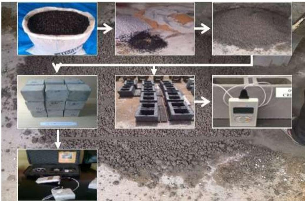
**Figure 1: Materials and Samples Preparation of Rubberized Blocks for Thermal Test**
