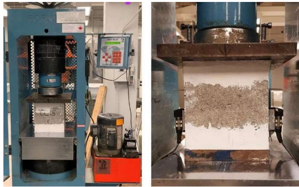
Figure 4: Compressive test setup
