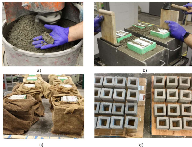
Figure 3: Blocks manufacturing process (a) Checking consistency of mix, (b) Compaction of concrete in moulds set on vibrating table, (c) Curing of the blocks, (d) Storing the blocks.
