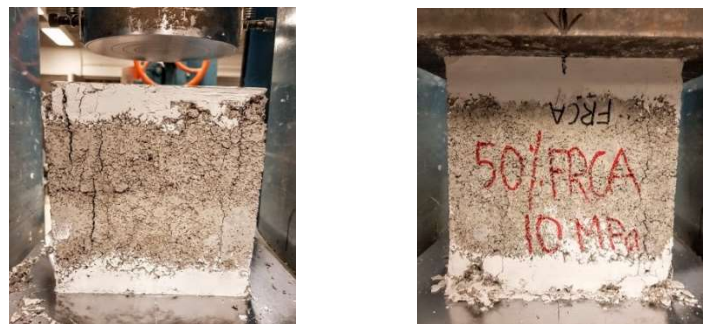
Figure 5: Typical failure mode: NAC Block (left) and 50% FRCA block (right)
