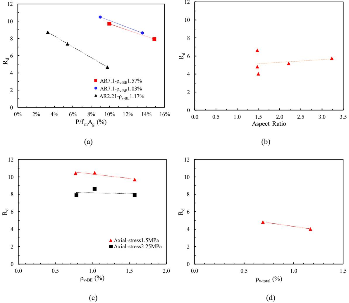
**Figure 3: Influence of design parameters on the ductility-related response factors**
