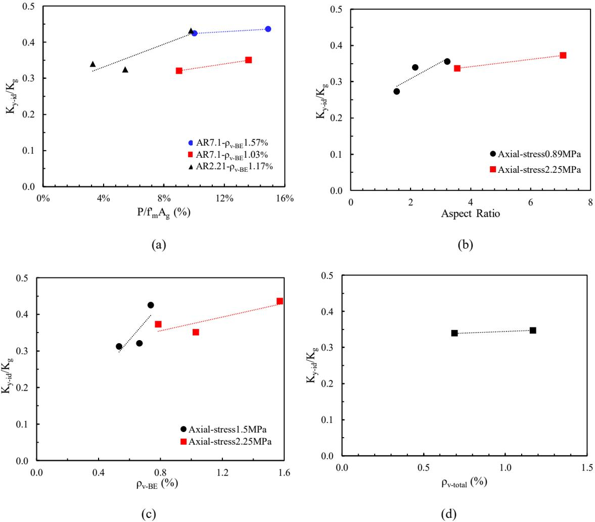
**Figure 4: Influence of design parameters on the stiffness degradation**
