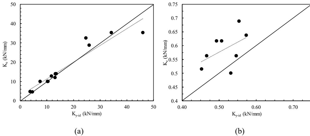
**Figure 5: Correlation between effective stiffness ( $K_e$ ) as calculated by CSA S304-14 and idealized yield stiffness ( $K_{y-id}$ )**
