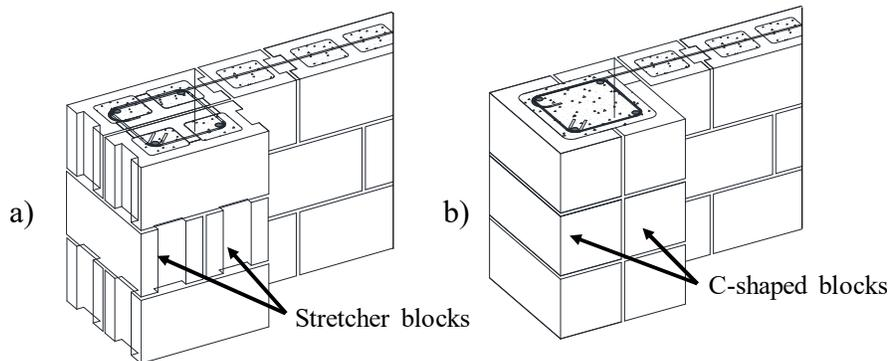
**Figure 1: RCM Shear Walls with Boundary Elements Built using: (a) Stretcher Blocks; (b) C-Shaped Blocks**
