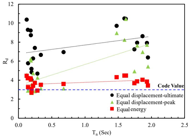
**Figure 2: Variation of ductility-related response modification factor with natural period of vibration**
