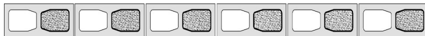
Figure 2: Example of typical grouting to increase the compressive strength of the wall, which leads to the mandatory fully grouted prism test
