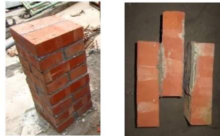
Figure 3: Masonry material test specimens: a) Prism; b) Triplet
