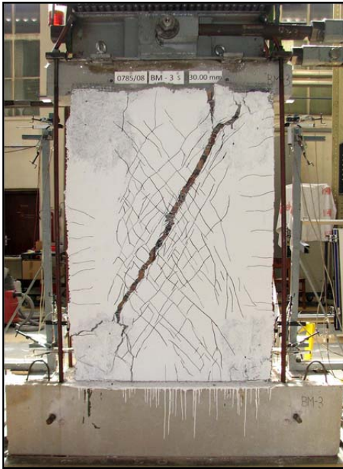
Figure 14: Brick Masonry. Diagonally Placed GFRP Grid Reinforced With Vertical Boundary Grid Strips [26]
