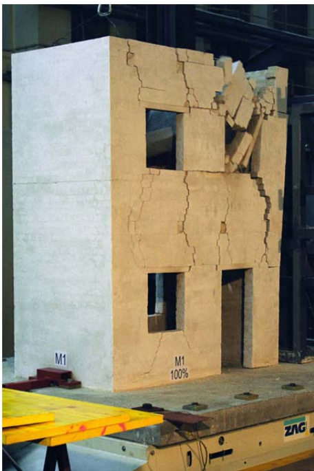
Figure 3: Upper Corner Failure and Separation of Walls of Model Without Wall Ties [19]
