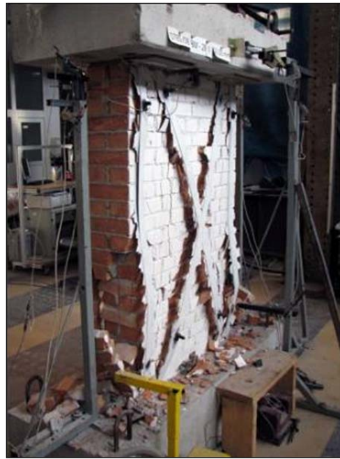
Figure 15: Brick Masonry. Delamination of CFRP Strips at Ultimate State [26]
