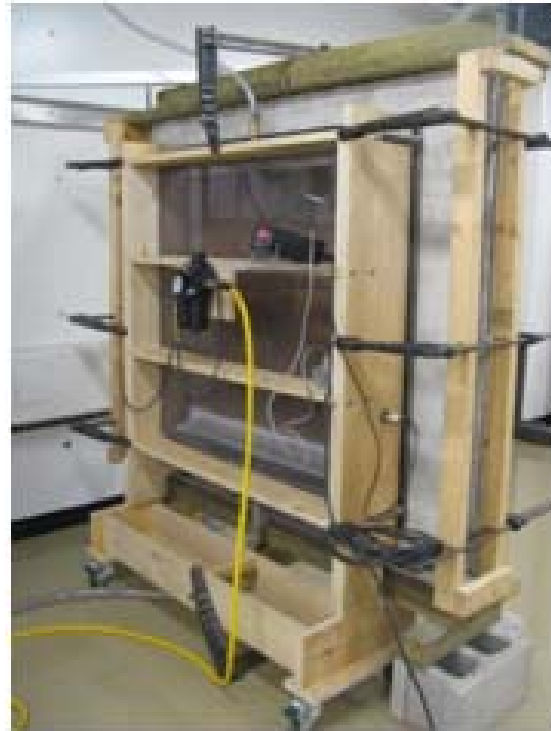
Figure 2: Wall Sample with Attached Test Chamber
