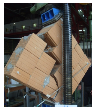
Figure 3: Different failure mechanisms from diagonal tests for: a) T1; b) T3; c) T5
