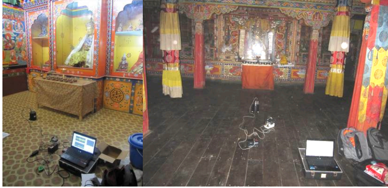
Figure 8: Experimental setup consisting of seismometer and data acquisition system at Enchey monastery and Labrang monastery
