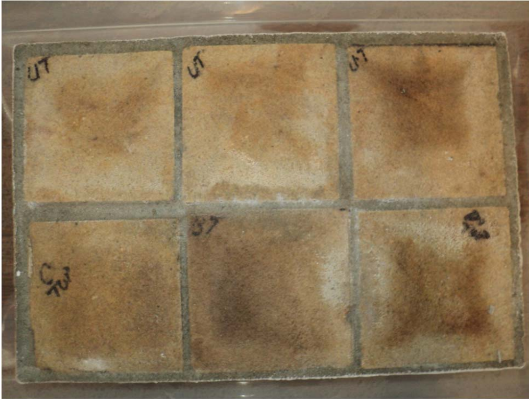
Figure 3: Brown staining on all pavers of Specimen A (approximately one week exposure)
