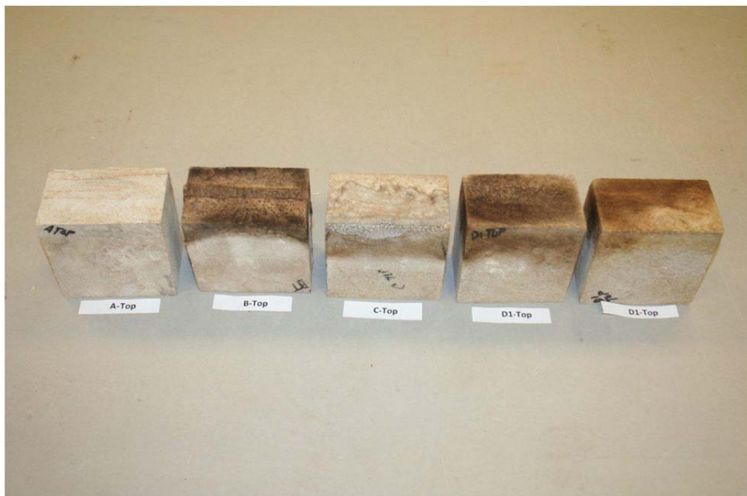
Figure 2: Four out of five previously installed paver samples effloresced
