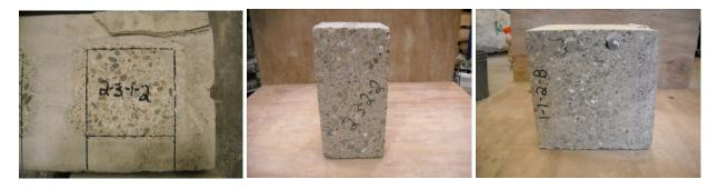
Figure 11: (a), (b), Side of Compression Specimen and (c) Consolidation Specimen with Steel Reinforcement
