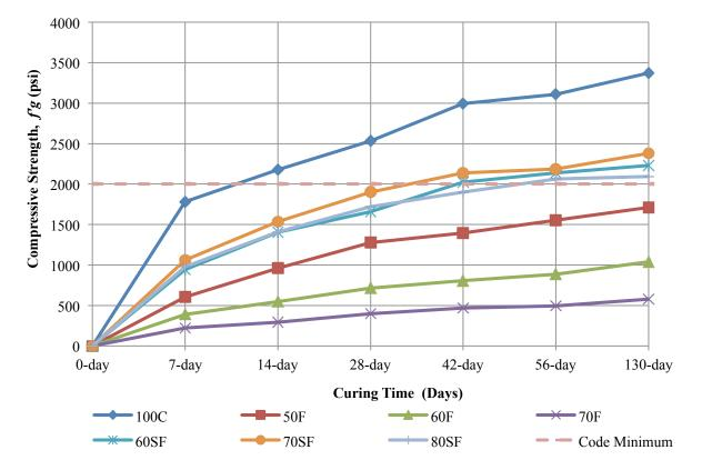
Figure 12: Average Net Corrected Compressive Strength of Grouts
