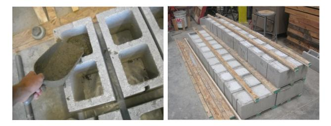
Figure 3: (a) Placing Grout into Cores of CMUs and (b) Dry Curing Grout Specimens
