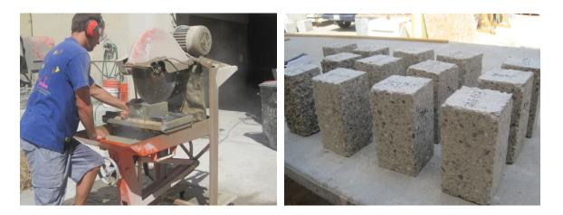
Figure 4: (a) Wet Saw Cutting Specimens and (b) Final Grout Compression Specimens
