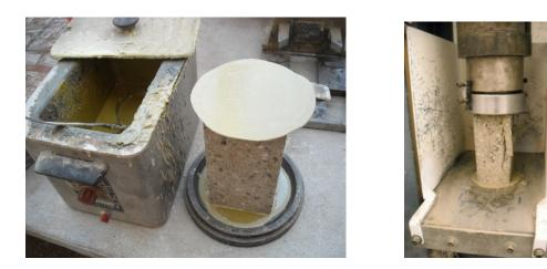
Figure 5: (a) Capping of Grout Compression Specimens and (b) Compression Testing
