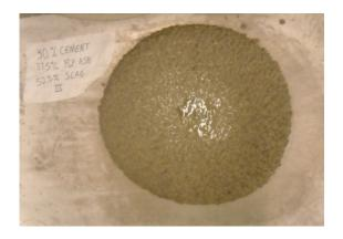
Figure 1: Slump Flow Picture of 70SF Batch 3
