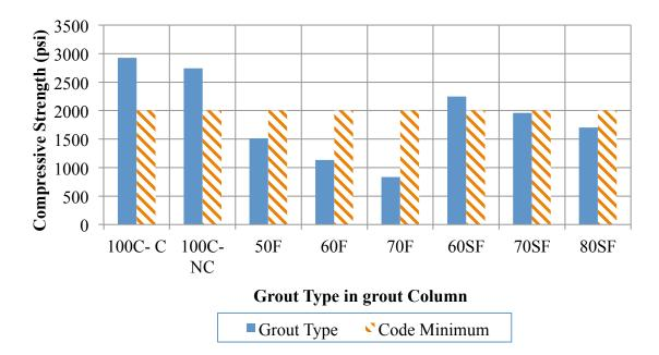
Figure 13: Average Net Corrected Compressive Strength of Grouts from Wall Grout Columns After 130 Days of Curing
