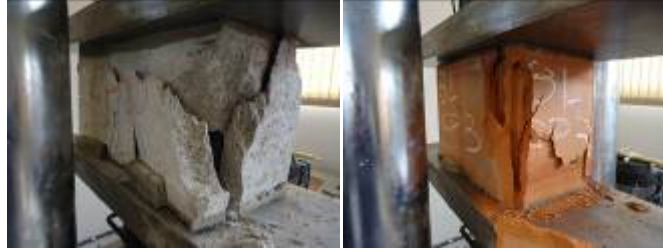
Figure 3 - Testing of concrete and ceramic block
