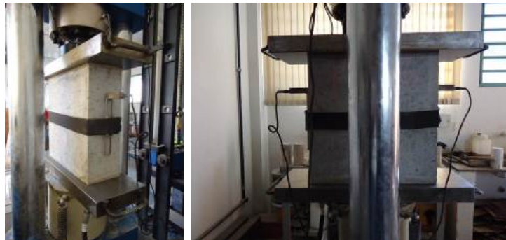
Figure 5 - Hollow Prism instrumented with transducers to obtain the displacements.
