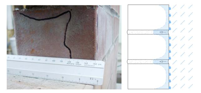
Figure 6: Test wall No. 2, water penetration after interval spraying of 5 l of applied water (left), schematic of water absorption during driving rain exposition (right)
