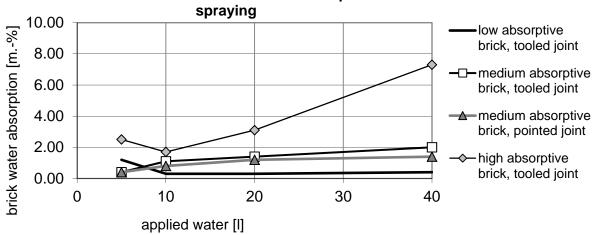
Sealed with 7.0 m-%-siloxane: brick water absorption at interval
