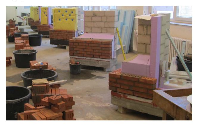
Figure 8: Test walls to investigate the watertight construction of ground-level door openings considering corners and edges
