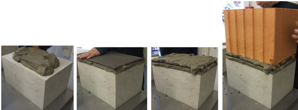
Figure 3: Production of Test Specimens with in Mortar embedded Damp-Proof Course
