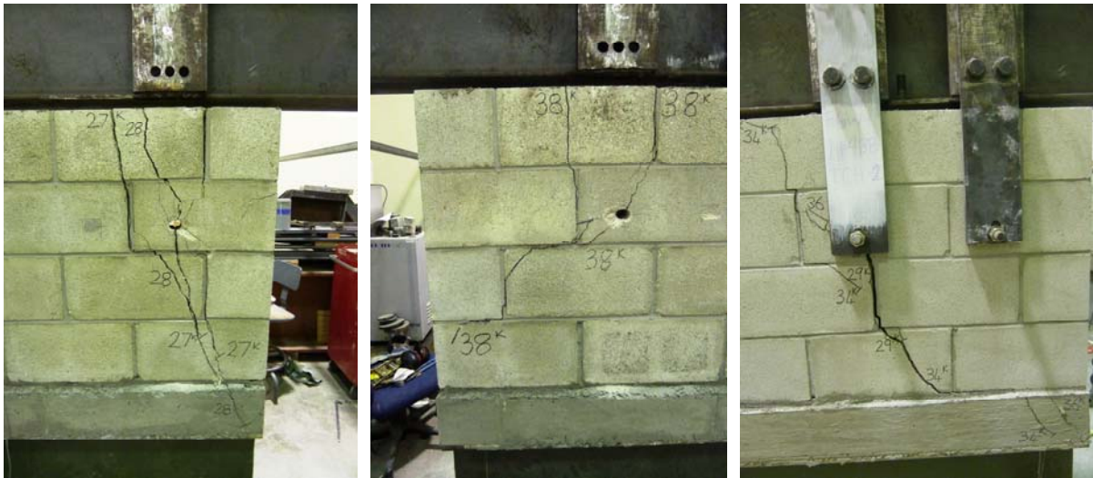
Figure 5: Specimen FGW-1#4BB Test 1 (left), Test 2 (center) and FGW-1#4BB-G Group test (right) after failure.
