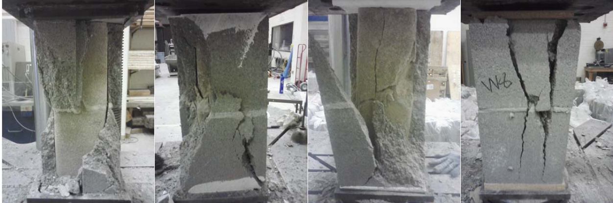
Figure 3. Failed Specimens: Neoprene, Gypsum, EPS, and Fiberboard Capping
