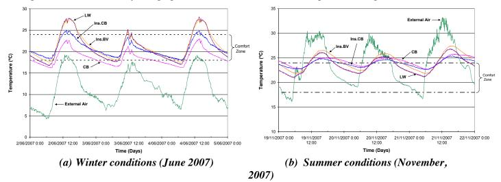
Figure 4: External and Internal Temperatures of Housing Test Modules Under Internal Floating Conditions (with North facing window)
