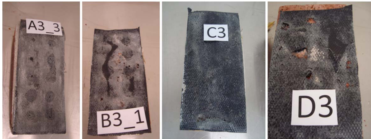
Figure 11: DPC Degradation under Highest Pre-Compression Level
