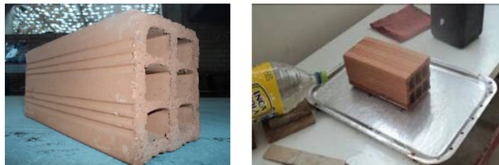
Figure 2: Horizontally hollow bricks and suction test
