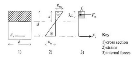
Figure 5: Stress and strain distribution in Eurocode 6 and BS 5628.
