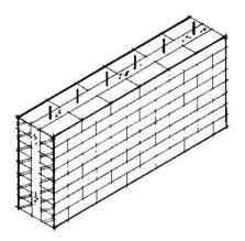
Figure 1: Grouted cavity masonry.
