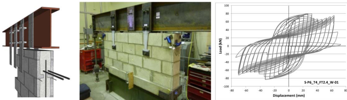
Figure 4. Testing of Fuse and Link Connectors at UHM
