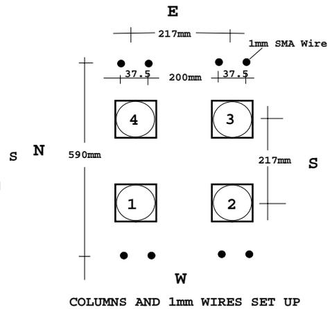
Figure 3b Location of the SMA wires
