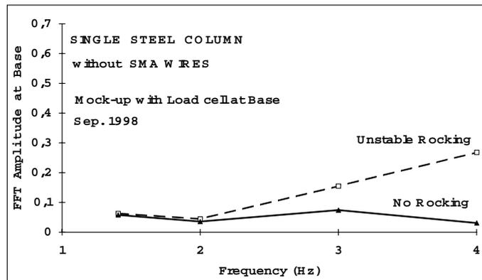
Figure 5a Single column response without SMA wires
