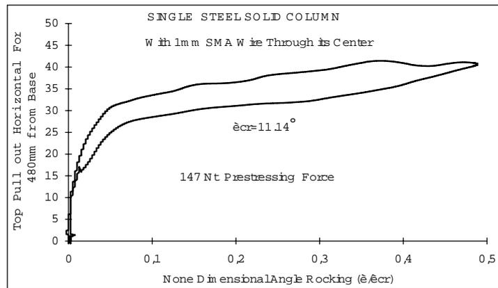
Figure 6a. Static pull-out response of single steel column with SMA wire
