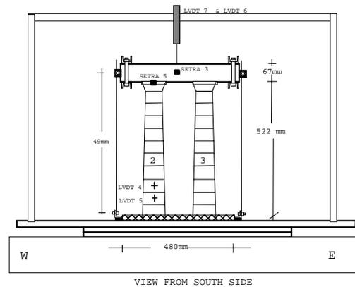
Figure 3d Four column colonnade. Testing arrangement transverse to the axis of the horizontal base motion.
