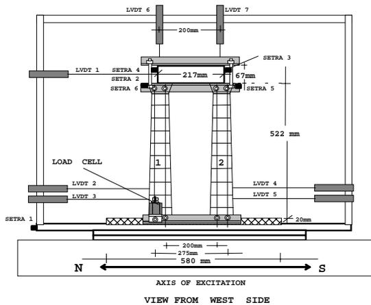
Figure 3c Four column colonnade. Testing arrangement along the axis of the horizontal base motion.
