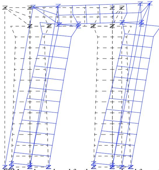
Figure 8. FEM mesh employed for the two steel and four-steel column colonnade
