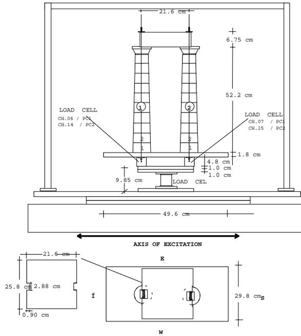
Figure 2. Two-steel column model colonnade
