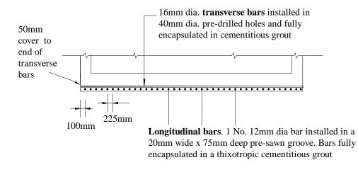
a). Cross Section through Arch Barrel
