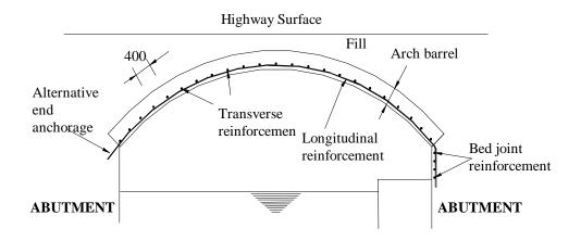
b). Longitudinal Section through Arch Barrel
