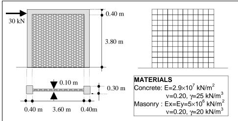
Figure 1. Geometry, mesh and materials characteristics of an one storey one bay frame
