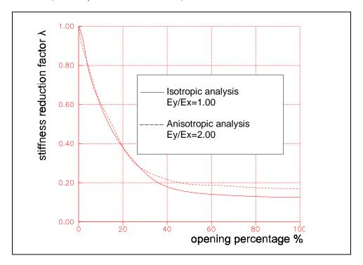
Figure 5. Stiffness reduction factor  $\lambda$  of the infilled frame in relation to the opening percentage for isotropic and anisotropic analysis
