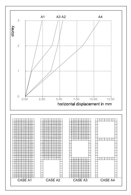
Figure 6. Storey displacements for different arrangements of the infill wall
