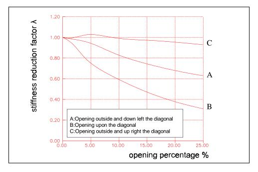
Figure 3. Stiffness reduction factor  $\boldsymbol{\lambda}$  of the infilled frame in relation to the opening percentage
