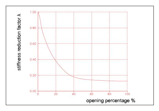
Figure 2. Stiffness reduction factor  $\boldsymbol{\lambda}$  of the infilled frame in relation to the opening percentage
