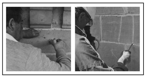
Photos 4 & 5: Using impact-echo (left) and fibre optics to investigate the condition of the inner core.
