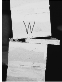
Figure 5 Ultimate limit state resulting from arising of a hinge in the mortar joint of masonry type CS-M 5,0 (MG II)
