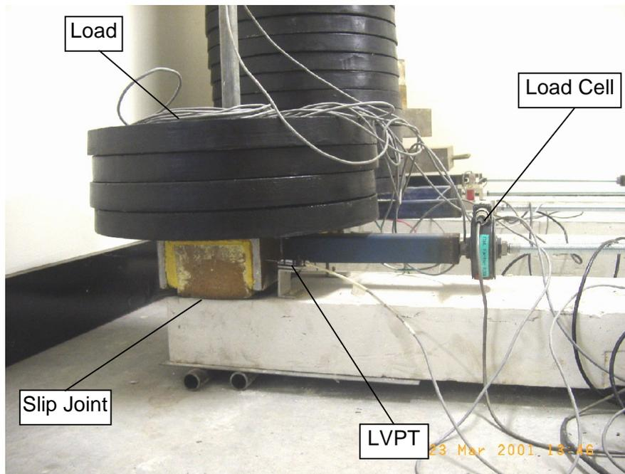
Figure 3. Instrumentation Set Up
