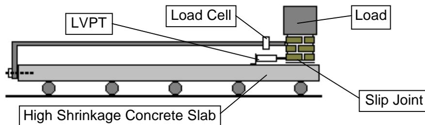
Figure 2. Schematic Rig Configuration for Shrinkage Tests
