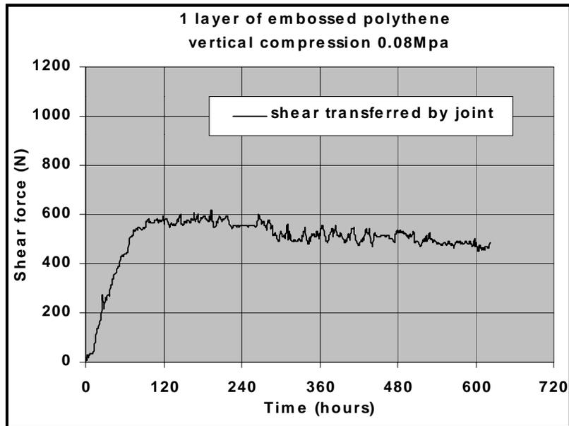
Figure 6. Shear Force Evolution in Joint Type 3
