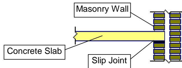
Figure 1. Slip Joint in Load-Bearing Masonry Wall
