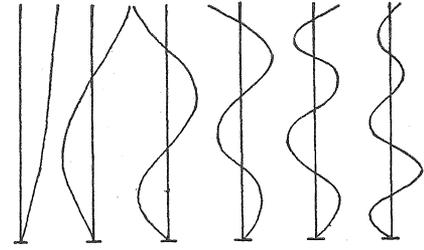
Fig. 5 First 5 Longitudinal Modeshapes
