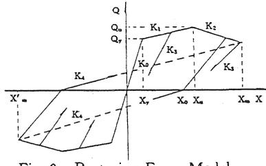
Fig. 3 Restoring Force Model
