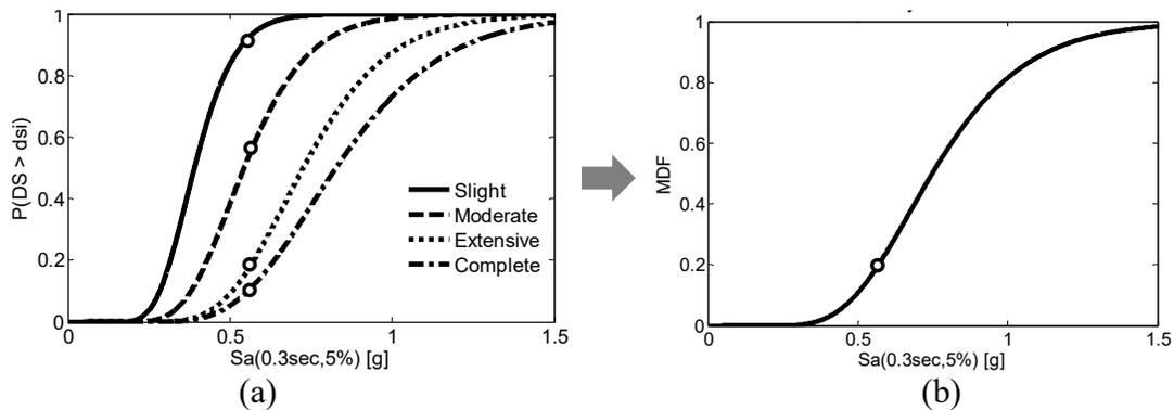
**Figure 1: Vulnerability analysis: (a) Seismic fragility functions and, (b) Vulnerability function. The dots illustrate the integration of the individual damage states from the fragility functions to obtain the respective vulnerability function**
