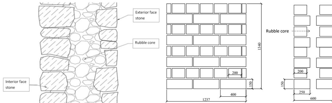
**Figure 5: URM wall cross-section and experimental test specimen**
