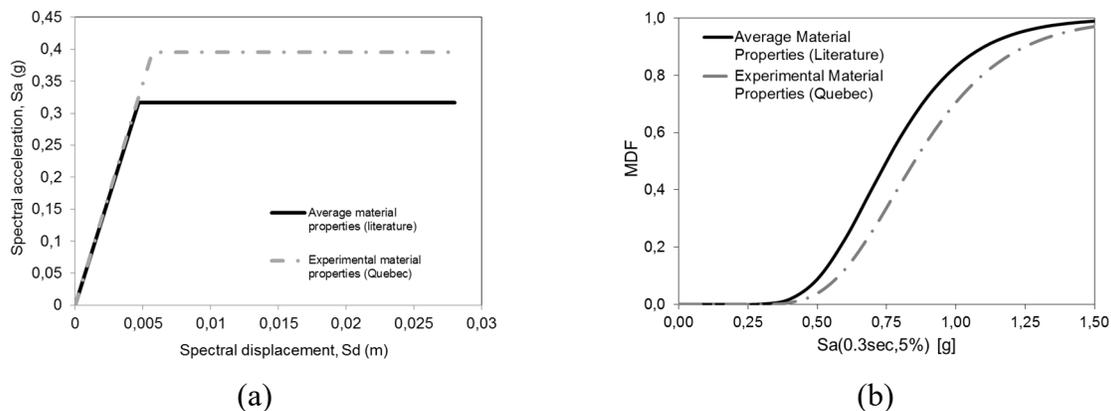
**Figure 7: Vulnerability functions: (a) Capacity curves, (b) Variation in yield spectral acceleration ( $S_{ay}$ ).**
