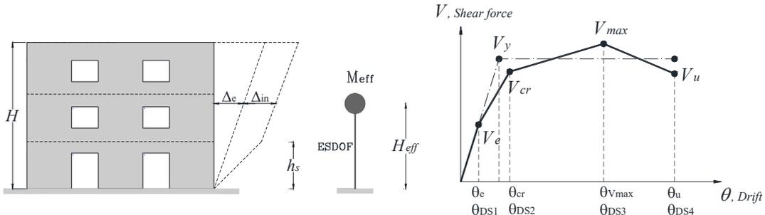
**Figure 3: Simplified model for computation of damage states**
