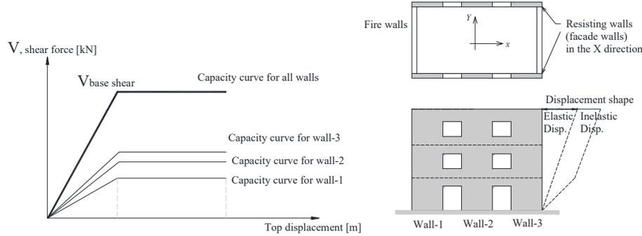
**Figure 4: Mechanical model for capacity curve evaluation of stone masonry buildings**
