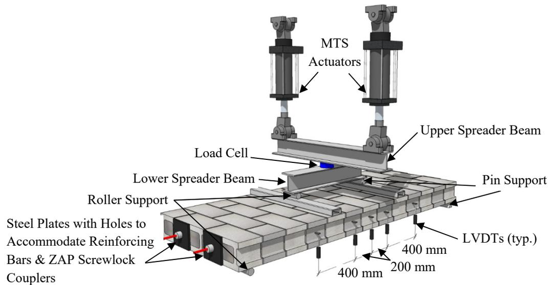
**Figure 4: Wall Splice Specimen Test Frame**
