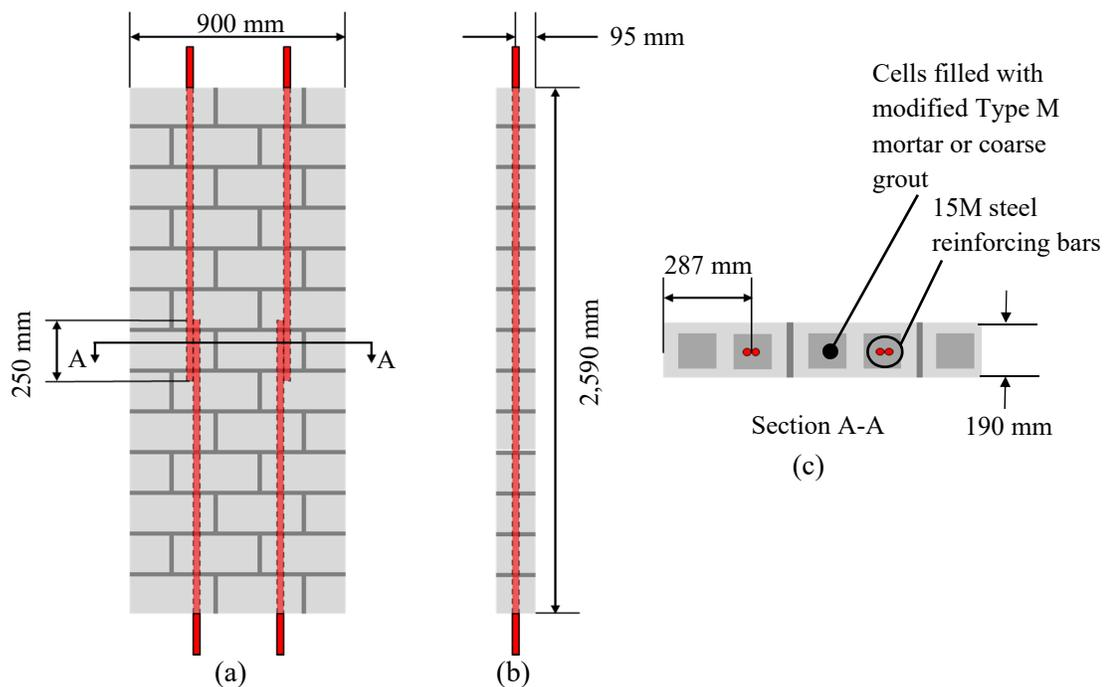
**Figure 1: Wall Specimen Details: (a) Front View, (b) Side View, and (c) Section Through Wall**
