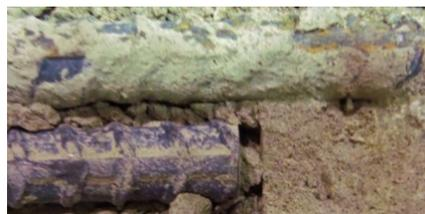
**Figure 6: Bar Slippage in Lap Splice Region**
