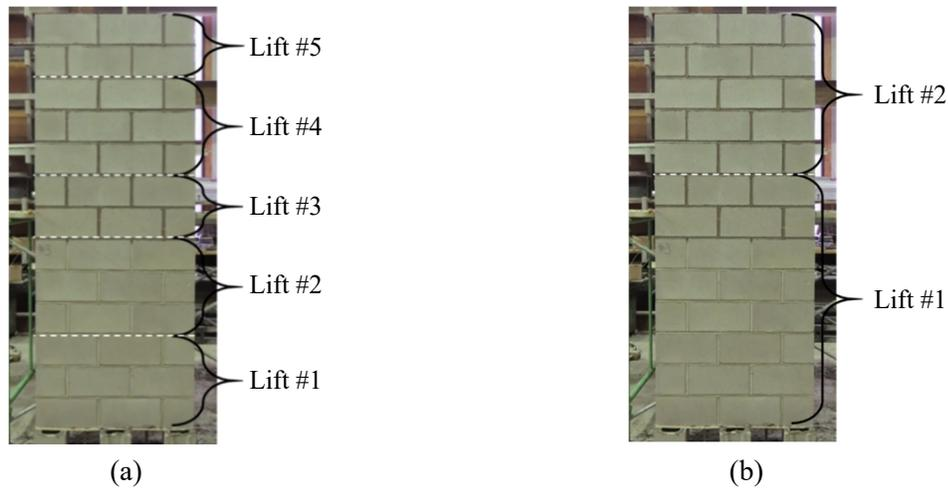
**Figure 3: Lifts in Wall Splice Specimens: (a) Grout-Like mortar, and (b) Code-Compliant Grout**
