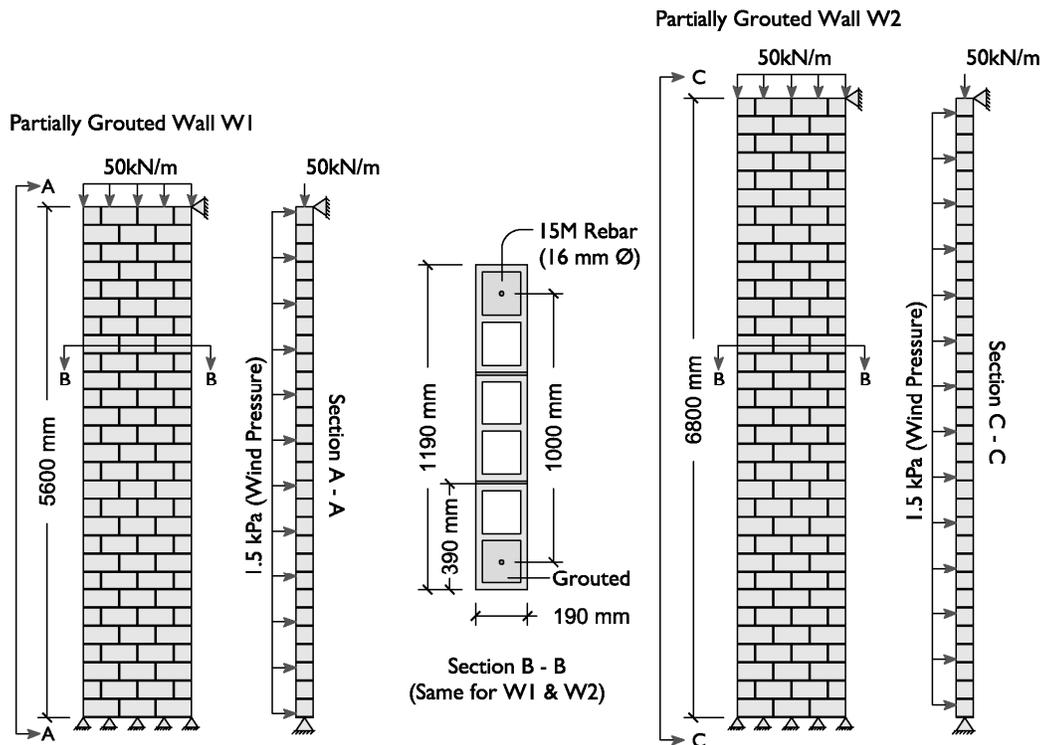
Figure 1: Partially Grouted Masonry Walls W1 (left) and W2 (right)
