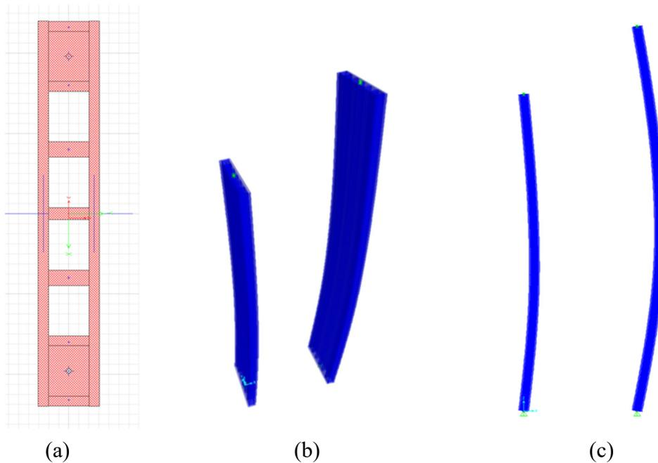
**Figure 2: SAP2000 Model: (a) Cross-section; (b) Isometric View; (c) Side View**
