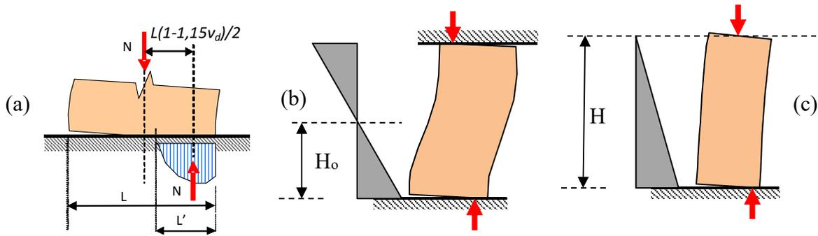
**Figure 3: Bending of a pier in its plane of action. a) Definition of Internal Moment and (b) Definition of the Effective Shear span  $H_o$  with reference to the moment diagram.**
