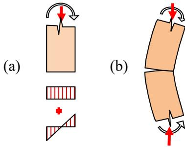
**Figure 6: Flexural strength calculation for out of plane bending. (a) Stress superposition at yielding, (b) Ultimate Flexural Strength**
