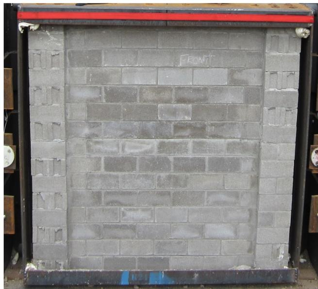
**Figure 2: Wall C-section steel support configuration.**
