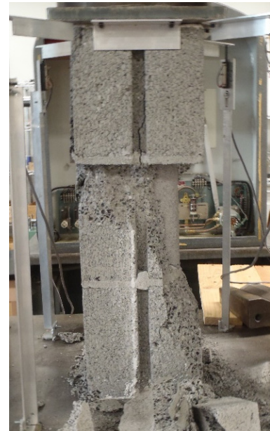
Figure 7: Failed FRG Prism
