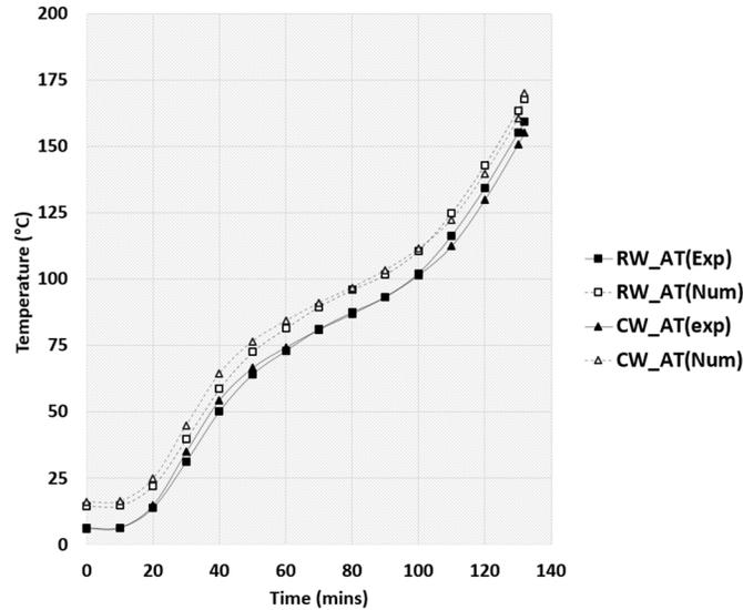
**Figure 4: Average temperature profile on the full wall (Raked and Control wall)**
