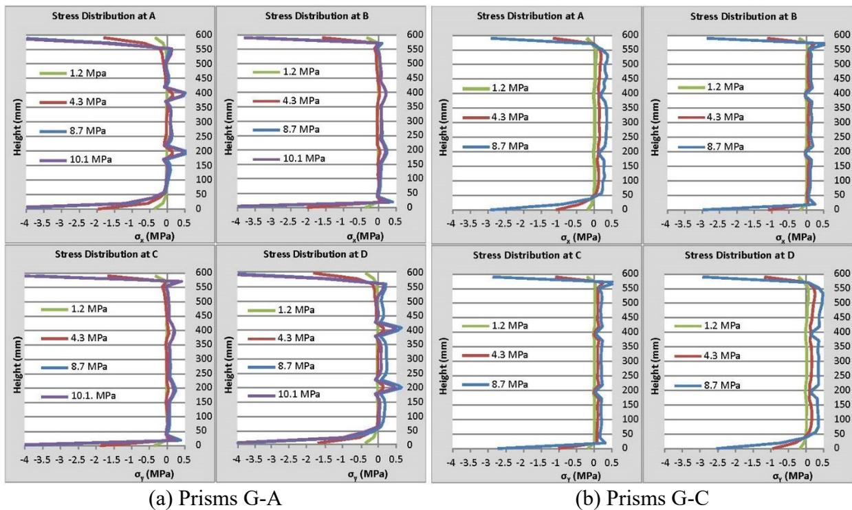
**Figure 9: Stress Distribution along Height of Prisms**
