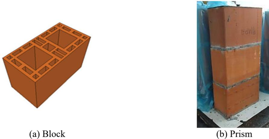
**Figure 1: Block and Prism Used**
