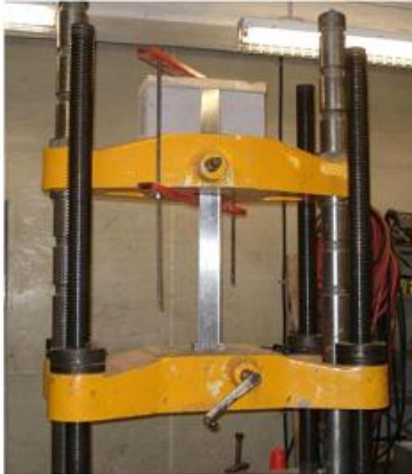
a) Testing capacity of tie anchorage (Test Setup)
