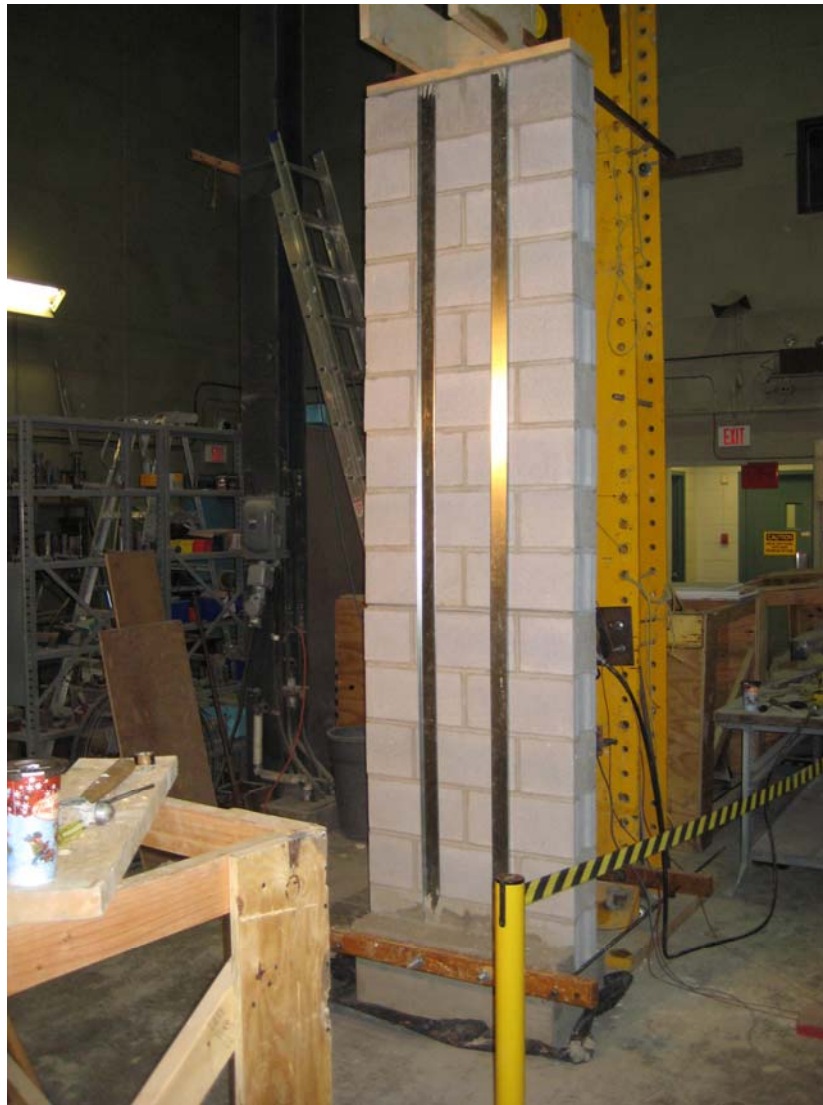
Figure 3: Wall 7 in Vertical Position for Lateral Load, Test No. 10
