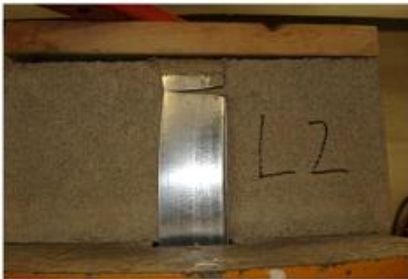
c) Typical steel failure at top anchorage
