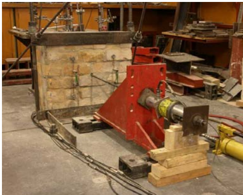
Figure 4: Pull-out connection test setup
