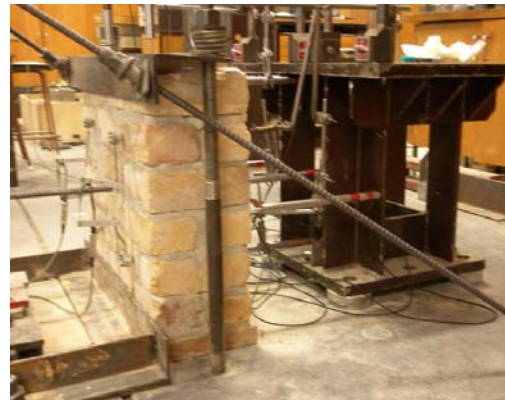
Figure 5: LVDTs to measure deflection
