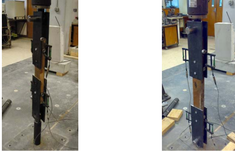
Figure 6: Typical specimen in testing apparatus: a) one bolt; b) two bolts
