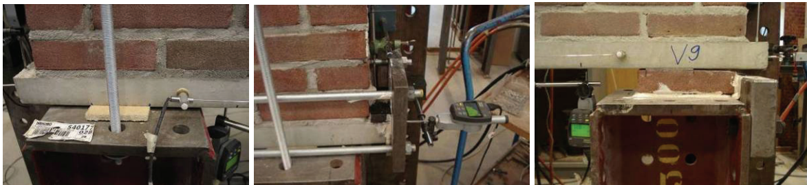
Figure 6: Supports in detail: a) roller, b) stiffened lintel and c) brick with felt.
