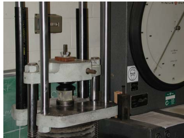
Figure 5: Mortar cubes: a) casting cubes in a mould, and b) compression testing
