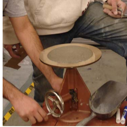
Figure 4: Mortar flow testing in progress
