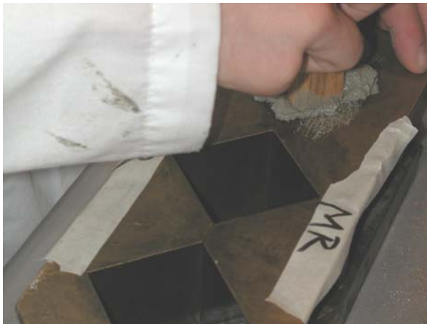
Figure 5: Mortar cubes: a) casting cubes in a mould, and b) compression testing
